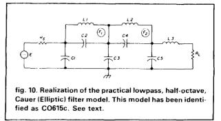
**Table 3** shows the calculated and practical values for all eight half-octave, low-pass filters used in the transceiver. The numbers in parentheses are practical values as used in the implementation. Silver-dipped mica capacitors with a tolerance of  $\pm 5$  percent were used throughout the networks. Breakdown voltages have been chosen at 250 volts.
